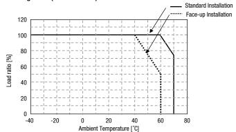
For Standard installation. -40 to 60°C (-40 to 140°F) at 100% load Derating -2.5% of load/K from 60 to 70°C (from 140 to 158°F)
